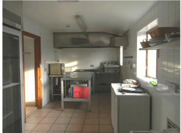
The kitchen was fitted c2005 with stainless steel furniture. It is known a push-through commercial dishwasher was once installed but has been removed, now a double deep sink unit exists here with a small hand washing bowl in the adjacent freezer area.
